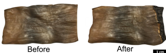
Fig. 5 Thin fragments of the coated material before and after exposure to flame
